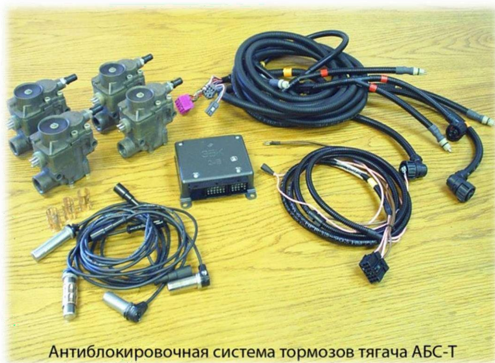
Fig.1. The anti-blocking system
